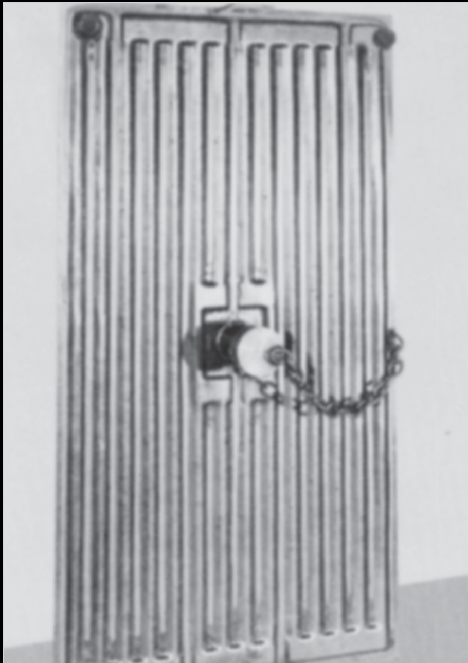
Water-cooled cover for electric furnace observation port
