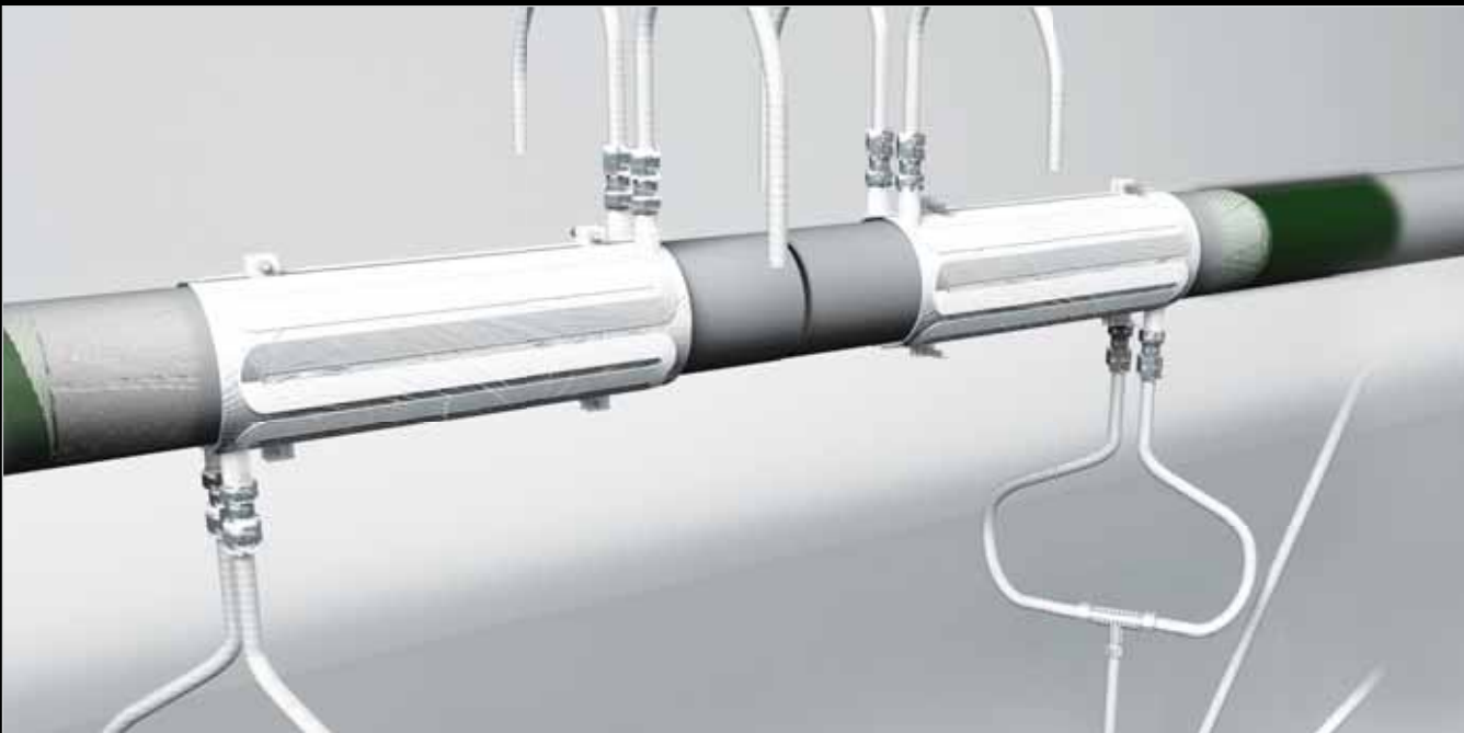
Using clamp-on PLATECOIL with cryogenic gas to freeze two plugs in a pipeline around a repair site
