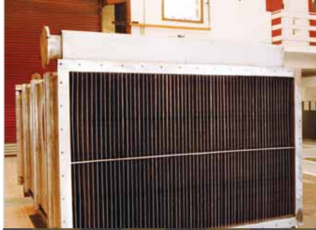
Waste heat recovery bank
