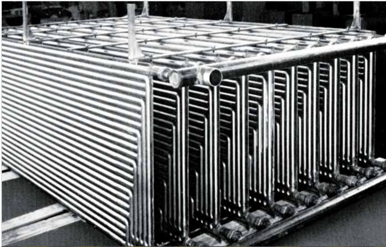
Bank for heating a product tank
