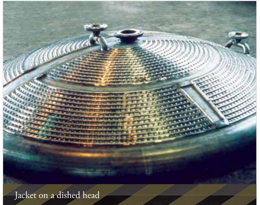
PLATECOIL embossings MIG welded to a heavy shell
