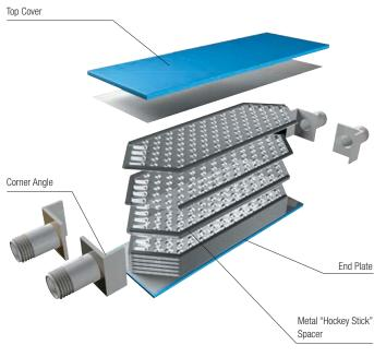
This exploded view of the welded MAXCHANGER unit shows the large number of dimpled contact points that provide maximum pressure resistance and heat transfer.
