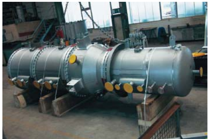
Spiral HEs configured as a three-stage overhead condenser.
