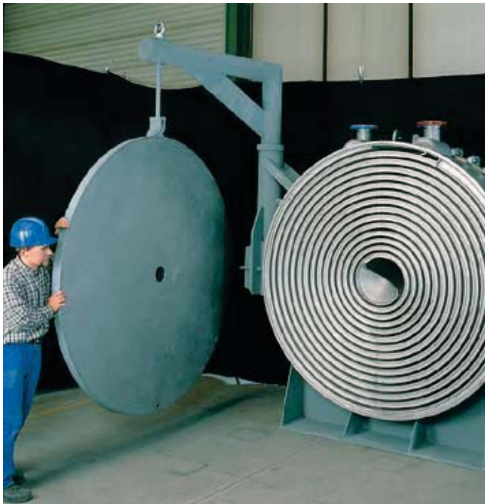
Sludge application with 431-ft 2 (40-m 2 ) surface area and 75-in. (1900-mm) diameter.
