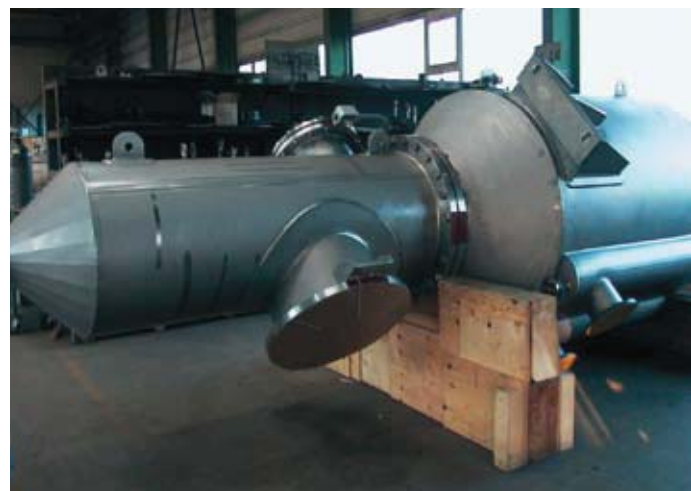
Spiral HE configured as a bottom condenser.
